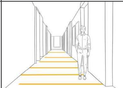
Embedded in the indoor floor (PVC/Silicone Material)
