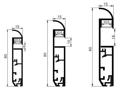
Light Source:2835 SMD LED strip,120leds/m Installation:Surface
